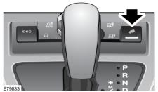
HDC can be selected at speeds below 80 km/h (50 mph). To select HDC, press and release the HDC on/off switch.
