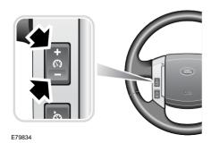
With HDC engaged, the speed of descent can be altered using the cruise control steering wheel switches. + increases the speed, and — decreases the speed.
